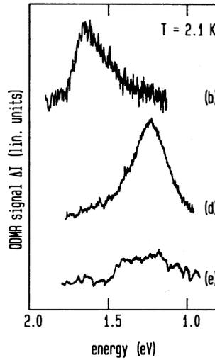
FIG. 3. Spectral dependence of the donor ODMR signals for (b) the starting material LEC GaP:S annealed in vacuum (800 °C, 1 h), (d) the irradiated sample which was subsequently vacuum annealed (800 °C, 1 h), and (e) GaP:Ge. Spectra (b) and (d) are measured at 2.1 K through a 1.5-m monochromator; spectrum (e) is shown for easy comparison and has previously been measured by one of the authors (see Ref. 6) on GaP conventionally doped with Ge.
