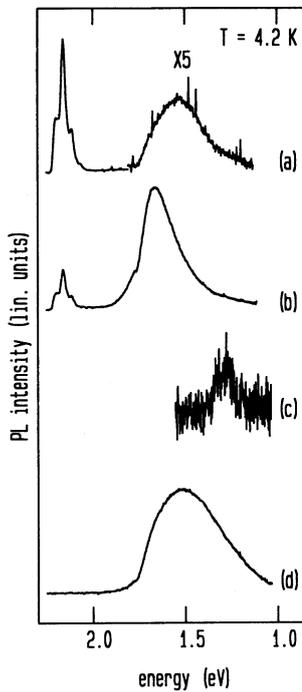
FIG. 1. Photoluminescence (PL) spectra of (a) the starting material LEC GaP:S, (b) the starting material annealed in vacuum (800 °C, 1 h), (c) the as-irradiated sample, and (d) the irradiated sample which was subsequently vacuum annealed (800 °C, 1 h). Spectra were recorded at 4.2 K through a 1.5-m monochromator within the range of the Ge detector using the 514.5-nm Ar<sup>+</sup> line to excite the samples.
