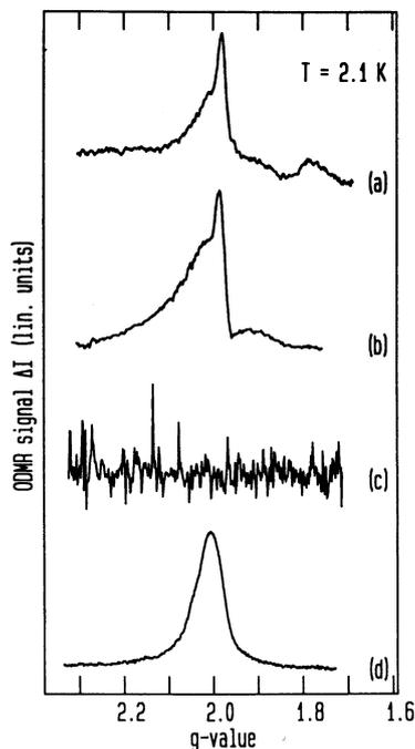
FIG. 2. ODMR spectra measured at 2.1 K of (a) the starting material LEC GaP:S, (b) the starting material annealed in vacuum (800 °C, 1 h), (c) the as-irradiated sample, and (d) the irradiated sample which was subsequently vacuum annealed (800 °C, 1 h). Changes of the total infrared emission ( $\Delta I$ ) under 514.5-nm Ar<sup>+</sup> excitation are plotted against the  $g$  value.
